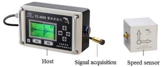
Figure 6. The measurement system of blasting vibration.
