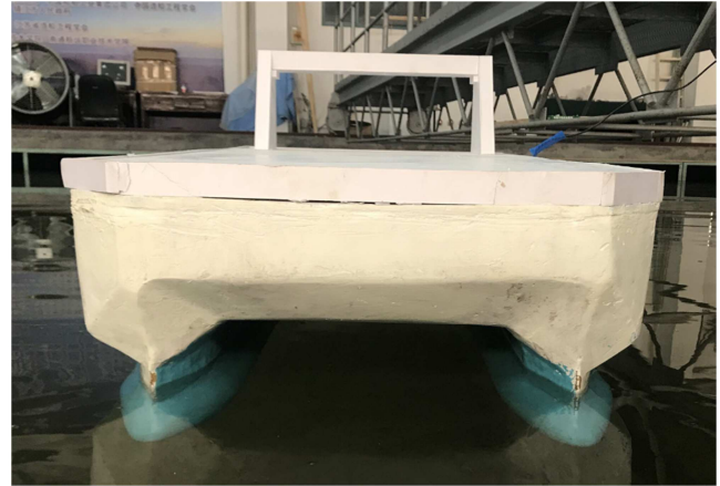
Figure 1. SWATH-USV model pitch test.
